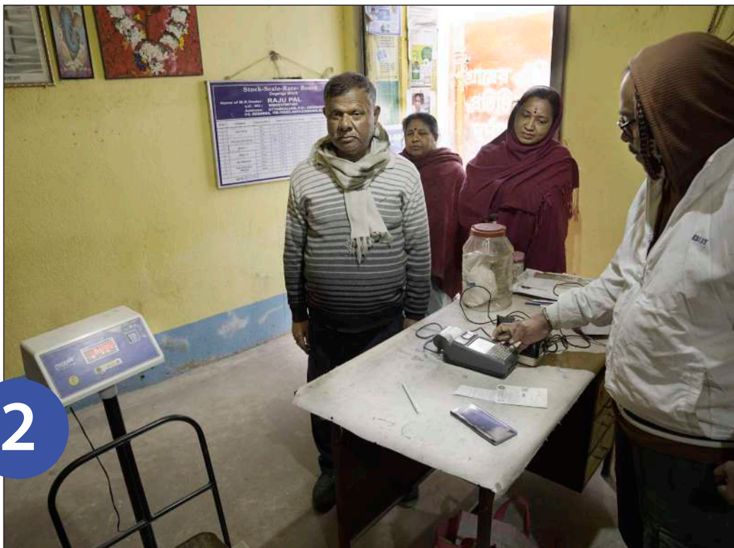
Scales are connected to the e-PoS device. A transaction can be processed only when the weight of the foodgrain is equal to the entitlement of the beneficiary.
