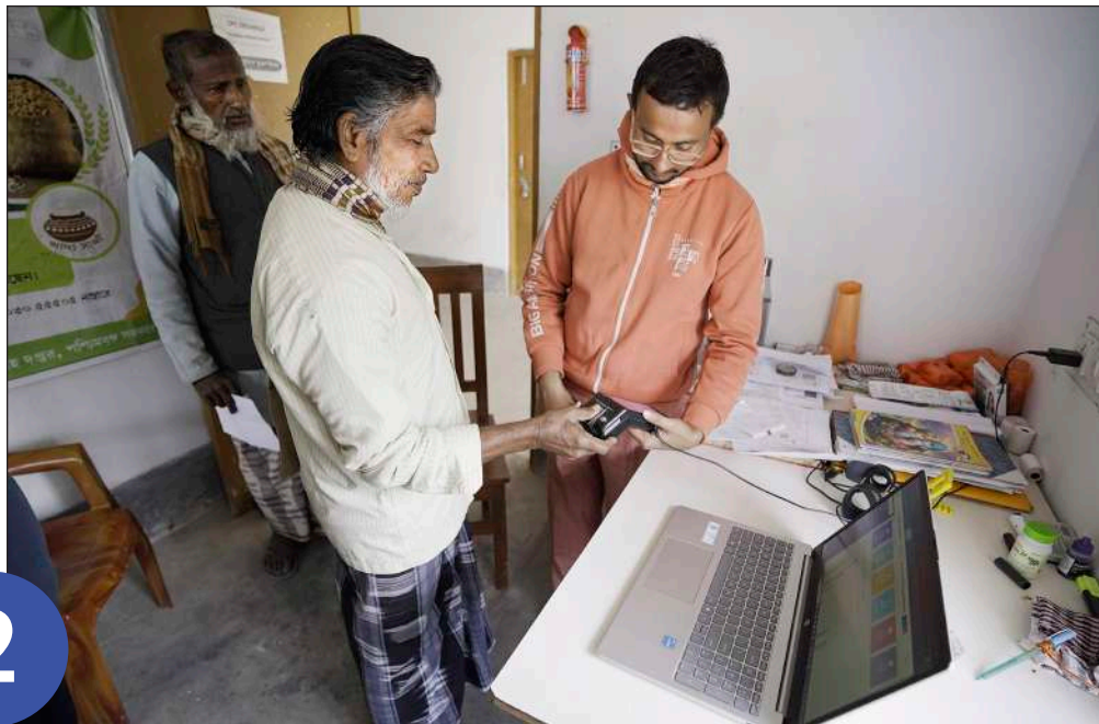
A layer of biometric authentication makes the process proof to tampering. The e-PoP (Point of Purchase) machine comes with a fingerprint and iris scanner.
